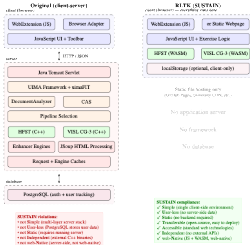
Figure 1: Architecture comparison showing the evolution from VIEW’s Russian module to RLTK. Parallel components share colors across both diagrams (e.g., green for NLP tools). Left: the original client-server design required a Java application server, the UIMA framework, C++ NLP binaries, and a PostgreSQL database. Right: the RLTK architecture compiles all NLP tools to WebAssembly and runs entirely in the browser, satisfying all SUSTAIN principles
