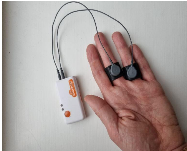
Figure 2: A GSR unit connected to a participant, ready for data collection.
